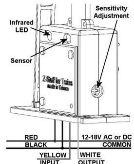
**TIME DELAY** - The time between aspects can be set from 1 to 60 sec. Hold the YEL & WHT wires together before power is applied. Turn on power (signal flashes 1/sec.) and hold YEL to WHT for desired delay. Remove WHT from YEL after the delay time you desire. Turn off power. When power is turned back on the delay you set will be the delay between each signal aspect indication. Check our website for applications and use of signals with our DZ-2500.
